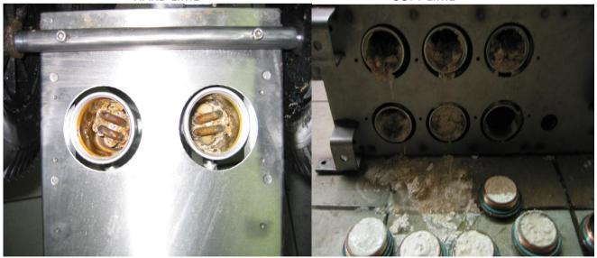
Soft lime goes away with water pressure. First try this. Hard lime requires chemical cleaning (DESCALING). DO NOT use sharp or hard objects to try and scrape off the scale.
